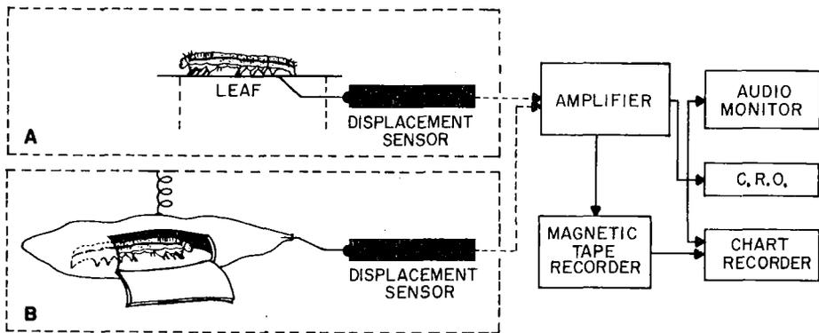
Fig. 1 Schematic of the components used in the recording of feeding activities of phytophagous insects with chewing mouthparts. A. system used with leaf feeders; B. system used with fruit borers.
